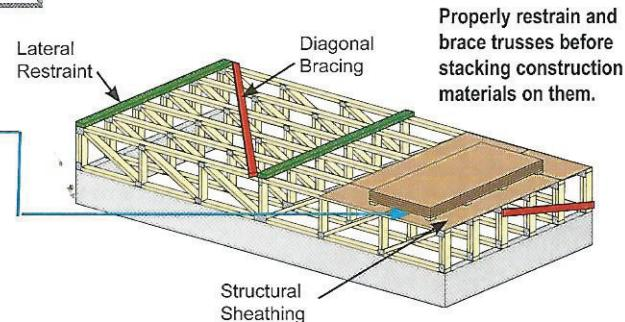
**DO** distribute loads over as many trusses as possible. Position stacks of materials flat with the longest dimension perpendicular to the trusses, as shown.
