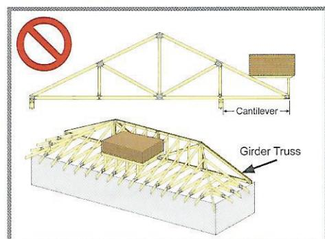
**DON'T** stack materials at locations that will produce instability, such as on cantilevers, overhangs or near truss-to-girder connections.
