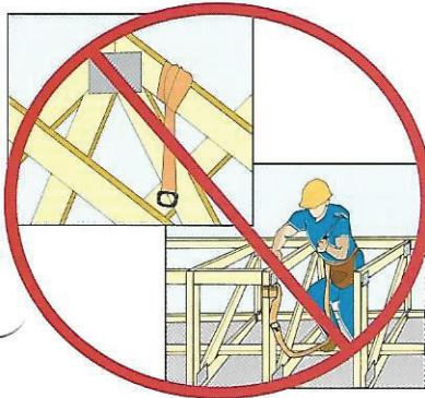
**DANGER** Any part of an inadequately braced or sheathed roof or floor truss system used as an anchorage point for any type of personal fall arrest system is dangerous and will increase the risk of serious injury or death.
